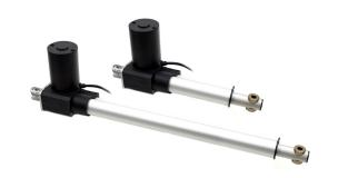
Compact and economic heavy duty linear actuator for the bigger projects, where it can be used for numerous purposes. The actuator moves with 20mm per second and stops automatically when fully retracted or fully driven out. This makes it easy to mount without having to us endstops or similar.
