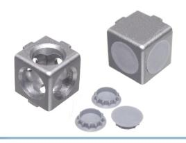
The corner joint is a small and solid bracket, for assembling 2 or 3 series 20 profiles in a corner. Threads are cut in to the end of the profiles, where after they are bolted through the bracket. The mountingholes are hidden with the included plastic caps.
