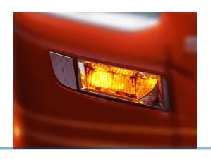
Emitters with 18 bright LEDs, specifically developed for the original Scania LED foglights. The emitters are available in xenon white, yellow and warm white, lights up the whole reflector of the foglights. The light is not blinding and works as position lights. The clever design allows you to fully keep the function of the foglight.
