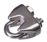
Solid clamp for locking one or two wires together. The clamp is locked by fastening the two nuts. The clamp is made from stainless steel A4.
