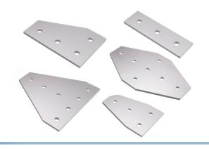
Extra strong brackets for 4040 profiles, milled out of 6mm aluminium, that is anodised. The holes fit M8 bolts. The different models can be used for various types of joints.
