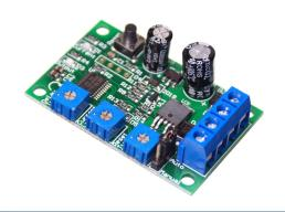
Smart protection against high current, that can be used for protecting motors, actuators and other similar current-variable units. When you block a motor or an actuator, it will use an extra high current, which very quickly can result in the motor overheating and be destroyed. This protection can prevent this, by shutting the power off.
