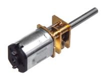
Incredible small gear-motor, type N20, that is only 10x12x24mm, with a 20mm long axle and Ø3. The motor is available with RPM from 100 to 1000.
