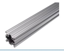
Large strong V-slot profile with dimensions 40x40mm. It has a high stiffness and can be used as a rails for heavy loads. There are 2 smooth V-slot tracks on each side, with a total of 8 tracks, where you can use V-slot wheels and mini-wheels.
