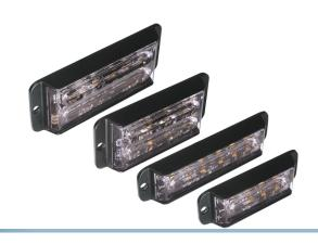
LED strobe with bright yellow 5W LEDs, that can be mounted on cars, trucks and motorcycle, and connected to 12V and 24V. The lamp has a solid aluminium housing, with large optical lens, that gives a wide light beam, and high visibility.
