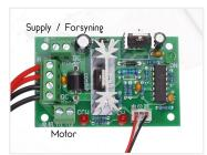
Compact speed regulator / motor controller for DC motors, with dial for speed and a 3 position toggle switch for chosing direction or stopping it. The speed can be regulated down to 5% depending on motor.
