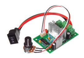
Compact speed regulator / motor controller for DC motors, with dial for speed and a 3 position toggle switch for chosing direction or stopping it. The speed can be regulated down to 5% depending on motor.
