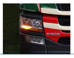
Complete LED light kit that replaces the original xenon white with, for example, yellow. The circuit board fits Scania +2016 trucks with halogen headlights. It has the same design as the original board, with the same connectors. Therefore, the replacement is quite straightforward.
