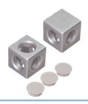
Smart and solid joint for screwing 2 or 3 profiles together in a corner. You cut threads in the ends of the profiles, where after you bolt these together from the inside of the bracket. Small taps go in to the profile, so that they cannot be teared loose. This gives you a very sturdy and durable joint, that has a high degree of stiffness.
