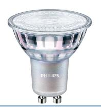
A dimmable LED from Philips with a classic look. It looks like a halogen bulb and behaves as such, but consumes only 3,7W or 4,8W, corresponding to a 35W and 50W halogen bulb respectively. LED bulb light scattering is 36 degrees and the GU10 halogen bulb is available with either a color temperature of 2700K or 3000K.
