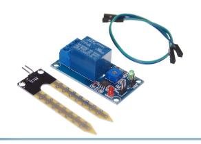
Sensor with controller that activates a relay, when the moisture falls under a defined value. The controller is easily adjusted with the small potentiometer.
