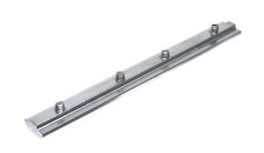
Strong solid alu-bar that fits in to 8mm series 30 slots. The bar is tightened between two profiles to join them. There are 4 pinol-screws that are used to fasten the bar.
