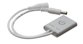
Dimmer that is mounted on the backside of wood or glass-sheets, where it can register touch through the material. It can be mounted on surfaces with up to 30mm thickness, for example tables, doors, etc. This makes it possible to do a completely invisible installation.
