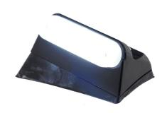
Top position lamps for the corners of Volvo FH trucks with a sleeper cab (CAP-SLP). A complete lamp consists of a Matronics Neon marker light, that is screwed on to a plastic housing, using the included screws. It is important that you seal between the lamp and the housing, specifically the hole for the wires, to prevent water ingress.
