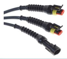
A simple splitter with a 2-wires cable and Superseal 1.5 plugs. It can be used to connect multiple lamps to one wiring harness. There is a 30cm wire on the inputs and on the outputs.
