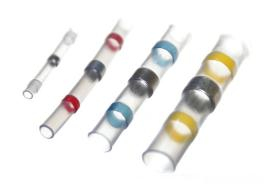
Solder-sleeves gives you secure and waterproof joints between wires. You can heat it until the solder melts and the crimp closes around the wires. The colored rings are glue that melts, and secures a waterproof joint around the wires.
