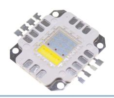
A very powerful high power LED with 4 color channels (RGBW / RGB + White), each shall be provided with 300mA-350mA. In each color channel, there are three strong LEDs in series. With a scattering angle of 140 degrees, it gives a very bright light. It has a life of 50,000 hours.
