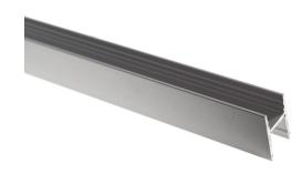
A nice annodized H-profile with space for LED stripes and plastic fronts at the top and at the bottom. The LED stripes are mounted, where after the fronts are clicked on. With the endcaps you close the profile and you get yourself a nice finish.
