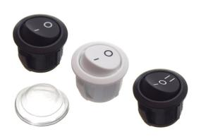
Switch with various functions, in black or in white plastic. It can be used for 12V, 24V and 230V. Panel-mounted in a 21mm hole. The panel-thickness can only be 0.7-3mm.
