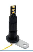
Flexible waterproof LED insert for figures and lamps, designed to be mounted in a 10mm hole and secured by tightening the bolt. The rubber blind nut makes installation incredibly easy, making it useful in hard-to-reach places. The blind nut expands and locks in the hole, and the assembly is therefore also waterproof.
