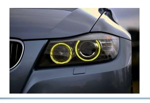
Complete set of light sources for BMW 3-Series 2009-2012 (E90, E91 Facelift / LCI) with LED angle eyes, to replace the white LED daytime running lights with yellow lights.
