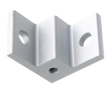
Corner bracket in solid aluminum, designed for mounting in the corner between two profiles. The side hole makes it easy to mount wheels or a foot. The bracket is installed with two M8 bolts.
