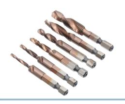
Combined drill and thread tap with a 1/4" hex shank compatible with a bit holder. The cobalt coating enhances the thread tap's strength, extends its lifespan, and increases hardness, making it ideal for demanding applications.
