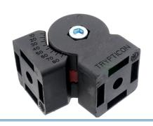
A robust three-part plastic arm that can be adjusted and locked in 5-degree intervals. Typically mounted between two profiles, it can be attached at the end or side of a profile thanks to the included 4 slot locks.
