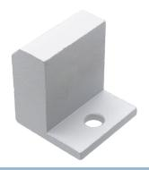
The aluminum bracket is attached at the end of series 30 profiles, where the large M8 hole (drawing B) makes it easy to mount casters / transpor wheels or a foot. Only a single M8 bolt and a T-nut are needed to secure it.
