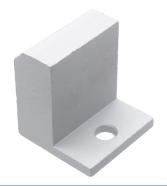
Aluminum end fitting with M6 hole, mounted at the end of a Series 20 profile. Can be used for a foot or transport wheel. Only a M6 bolt and T-nut, or hammer bolt and nut are needed for installation.
