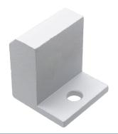
Aluminum bracket that screws into the end of a Series 40 profile. The large block has an M12 thread at the bottom (drawing B), for example, for a foot or for casters / transport wheels. You need an M8 bolt and a track-nut, or a hammer-bolt and a nut to fasten it to a profile.
