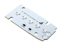
LED light source replacing the original ones in the reading lights in the ceiling of MAN TG 2023+.
