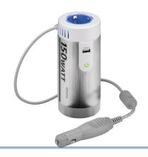
A voltage inverter that converts 12 V DC to 230 V AC, so that you can connect regular 230V appliances to a car, for example. Max power is 150W at 0.65A at 230V. There is also a standard USB plug that can be used for standard USB units. Max. USB current is 2.4A.
