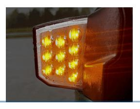
Simple adapter for the indicators above the headlights. Inserted between the original wire harness and the lamp, the last wire is connection to position lights.
