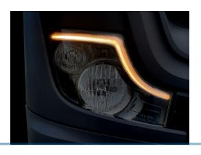
Complete LED DRL conversion kit for Mercedes Actros 2020 and the facelifted from 2023 and forward. Allows you to change from white DRL to eg. yellow. The xenon white emitters can also be used if the original are defective. The emitters have LEDs for both indicators and DRL.
