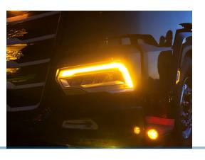
Complete LED DRL conversion kit for DAF 2021 and forward. Allows you to change from white DRL to eg. yellow or warm white. The xenon white emitters can also be used if the original are defective. The emitters have LEDs for both indicators and DRL.
