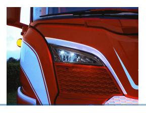
Emitter with 6 bright LEDs, for supplemental position lights in the high beams under the windscreen. Mounted on top of the original emitters.
