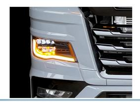
Complete set to convert the original xenon-white DRL. The set consists of two boards and thermal paste. There are 8 powerful LEDs on each board, newest generation of high power 5W LEDs from Edison. The brightness is equivalent to the original.
