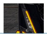
Complete set LED emitters for retrofitting your Volvo FH5, FM5, or AERO with amber DRL, or simply for replacing your emitters if one of the original breaks. These fit Volvo FH5, FM5, and Aero from 2021 and forward. There are in total 8 high-power LEDs per set with an output that is equivalent to the original.
