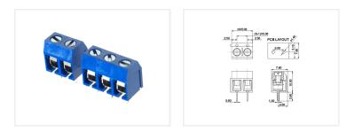
Screw terminals for through hole mounting in PCBs. 5mm pitch, 0.6mm pins. Available with 2 and 3 positions, that can be connected in a longer row.
