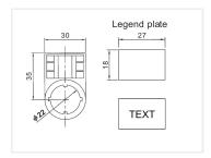
Holder in plastic for marking of buttons, and various labels, such as start, stop, up down. The waterproof nameplates are easily pushed down in to the holder, where they stay put.
