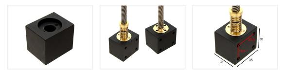
Housing in aluminium for M8 trapez nuts. Nut is mounted with 2 x M3 screws, housing is mounted with 4 x M4 threaded holes in the bottom.
