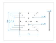
Standard Vesa monitor bracket in solid anodized aluminum. Can be mounted directly on profiles, on bracket and arms. You need M4 bolts for mounting the plate on the screen, and possibly also spacers, washers or nuts.
