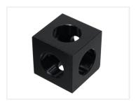
Solid corner in aluminium for joining 3 pcs of 20x20 V-slot profiles. It is bolted on with M5 low profile bolts in the ends of the profiles. Also called cube-corner in the v-slot system.
