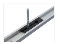
Slider in plastic, that locks itself in the profile when the bolt is fastened. This is typically used for clamps in fixtures and jigs. As it can be put directly down into the track. The special bolt needed needs to be bought separately, as it is available in various lengths.
