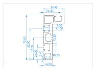
Fence profile that fits with the fence bracket, and glider with adjustable angle. Used for positioning and moving parts in the machine. In a table saw this would be used for the sled, and in a router, this would line up the parts being fed through.
