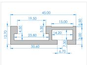
Standard profile with space for built-in tape, that can be used for positioning and measuring parts and fixtures. It is typically used with other profiles and accessories, eg. end-stops and fences. The profile has the same dimensions as the standard profile, but is 45mm wide.
