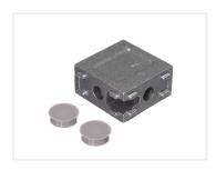
Solid 90-degree aluminium bracket for joining two 1530 profiles. The profiles with M6 threads in the center holes are bolted on to the bracket, and the included covers are placed in the holes.
