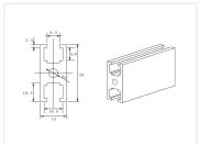
Strong profile that is intended for lids, doors and other parts that demand high stiffness. The profiles has tracks on the slim sides, and completely blank on the others.
