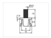
Cover strip with 10mm long  $\emptyset$  0.2mm brushes, that fit 8mm tracks, such as series 30 and 40 tracks. The brushes can be used for tightening, clean, guide and fix.
