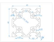
Large strong V-slot profile with dimensions 40x40mm. It has a high stiffness and can be used as a rails for heavy loads. There are 2 smooth V-slot tracks on each side, with a total of 8 tracks, where you can use V-slot wheels and miniwheels.
